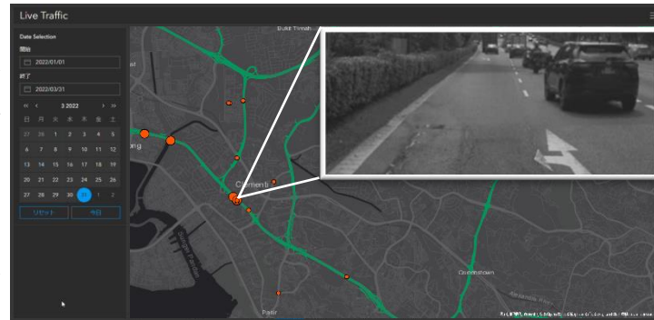
Potholes detection (dashboard)
