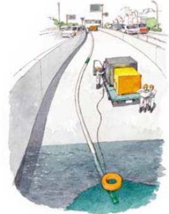
Drainage of Flooded Water at Under-path
