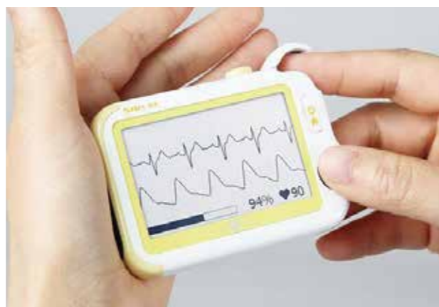
Daily Check mode which can take recording of ECG and SpO2 at the same time.
