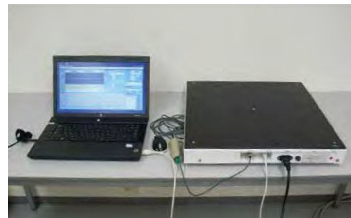
Medical Sole Tester; Equipment to measure original tactile stimulus (misalignment of skin surface) easily and sensitively
