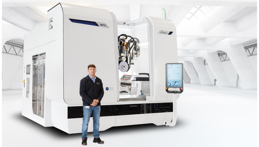
The MFP-51 (5-axis grinding center) is particularly suitable for applications in the turbine sector (aviation and energy). © Mägerle AG Maschinenfabrik
